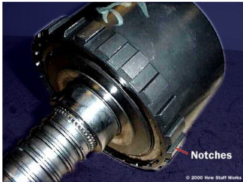
The output of the transmission: The square notches are engaged by the parking-brake mechanism to hold the car still.
