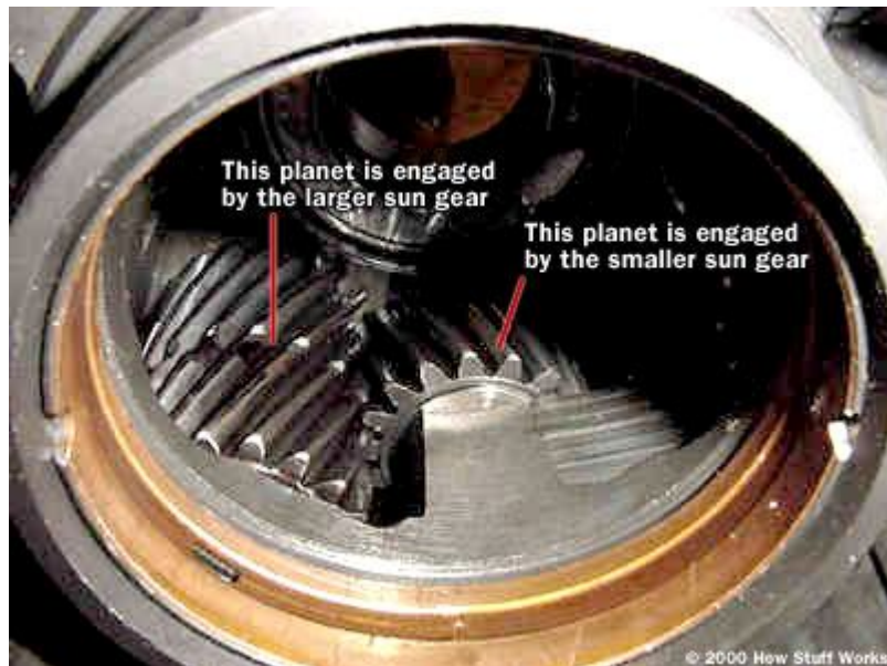
Inside the planet carrier: Note the two sets of planets.
