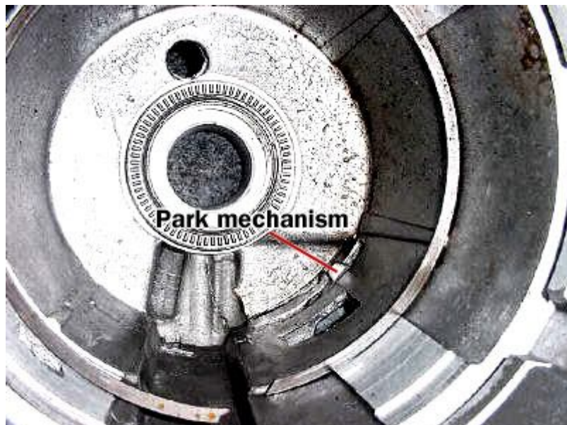
The empty housing of the transmission with the parking brake mechanism poking through, as it does when the car is in park
