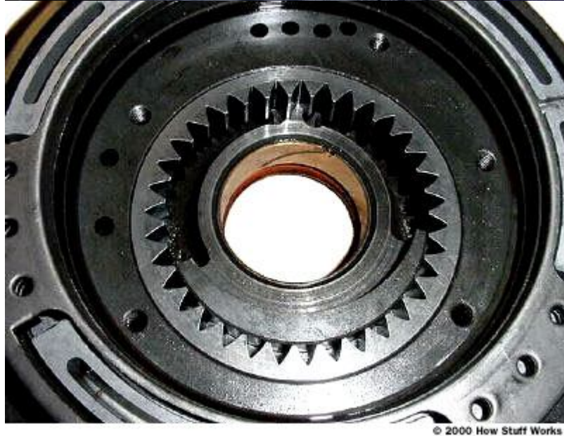
Gear pump from an automatic transmission
